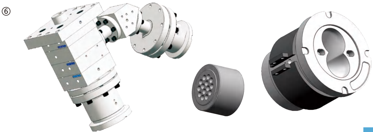
6. Feedblock Adapter + Multihole Bush a. Feedblock can solve the problems of high pressure on downstream, uneven co-extrusion layers and short running time. b. Adapter with temperature control device can solve over-temperature problem. c. Multihole bush can promote plasticization and save formula cost and solve color difference and board surface lines problems.
